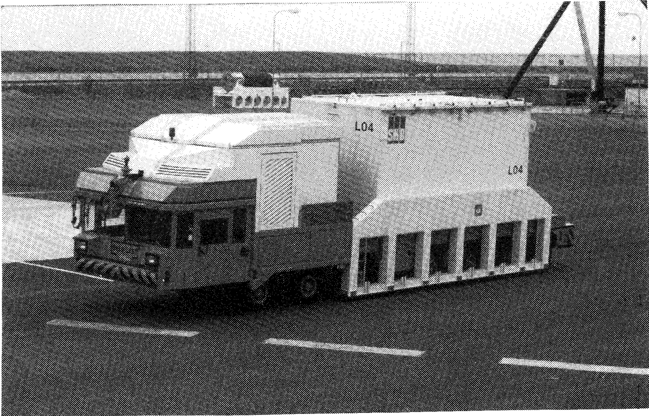
Figure A2.2 Terminal vehicle at SFR with radiation-shielded transport container for intermediate-level waste.
